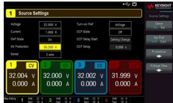
Figure 7. E36441A provides OVP, OCP, and OTP protections
