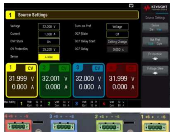
Figure 6. E36441A offers four-wire remote sensing for more accurate power delivery
