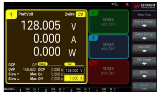
Figure 3: Increase output voltage with E364SNP kit.
