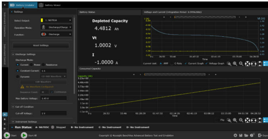
Figure 9. BV9210B enables you to choose various discharge mode options (constant current, power, resistance, and dynamic current discharge)
