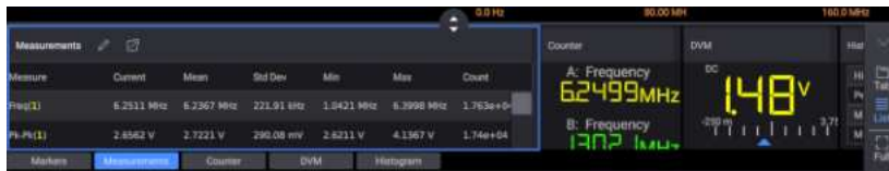
Figure 4 Listed windows in Results area
