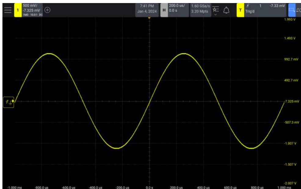
Figure 32 128 Averages used to reduce random noise
