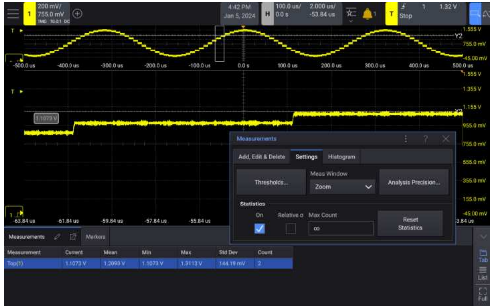
Figure 38 Isolating area for Top measurement
