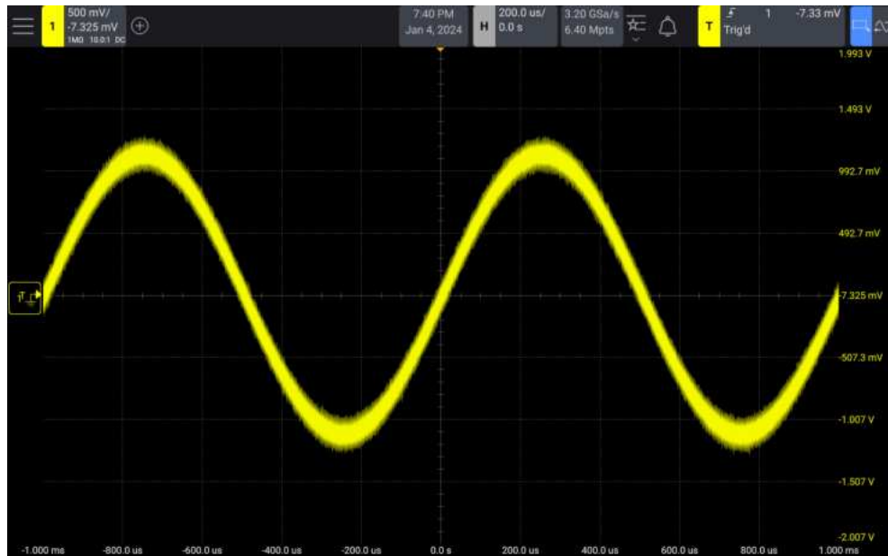
Figure 31 Random noise on the displayed waveform
