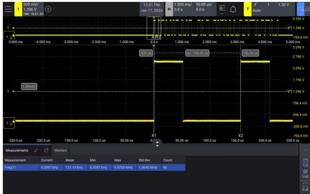
Figure 40 Isolating an event for Frequency measurement
