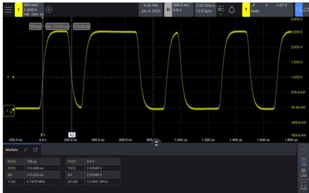
Figure 36 Measuring pulse width with markers
