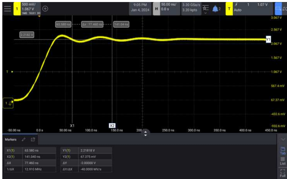
Figure 34 Markers measure frequency of pulse ringing
