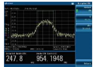
Power suite – Occupied bandwidth
