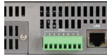
Figure 4. Digital control port on the rear panel
