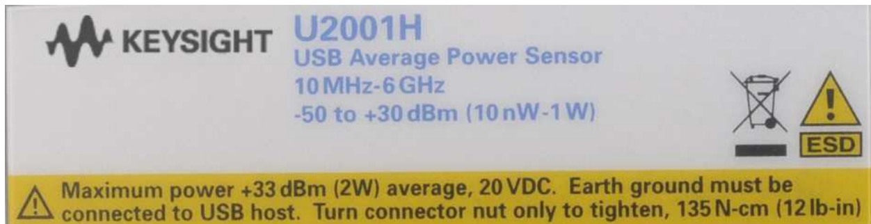
Figure 1. Front label of Keysight U2000 Series USB power sensor
