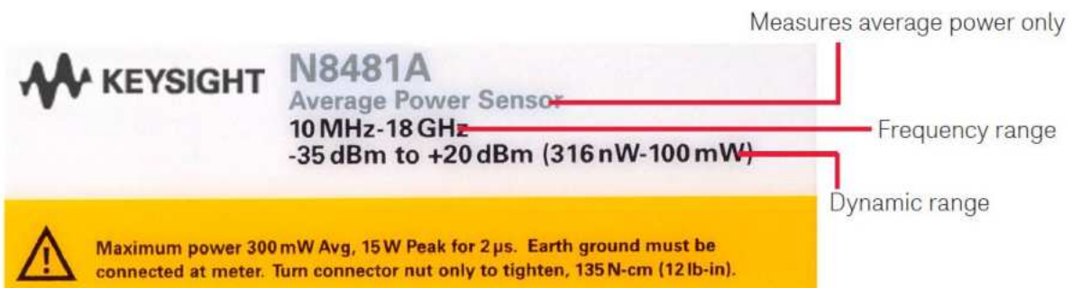
Figure 5. Front label of a thermocouple average power sensor
