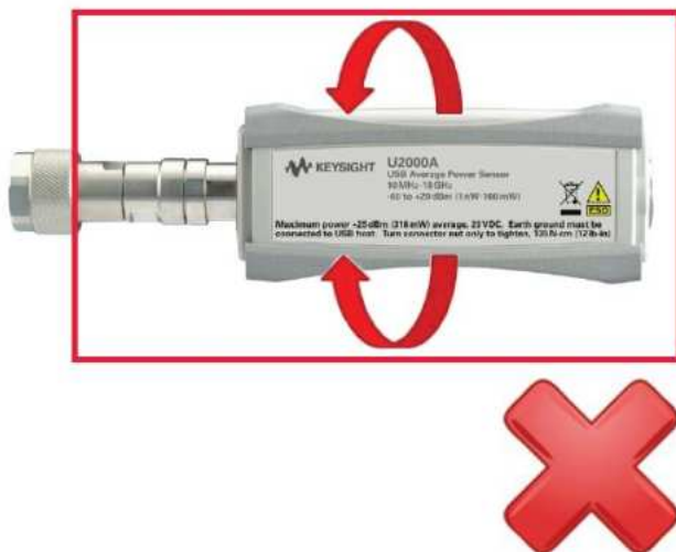
Figure 6. Do not turn the power sensor body
