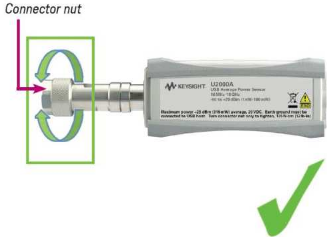
Figure 7. Turn only the connector nut
