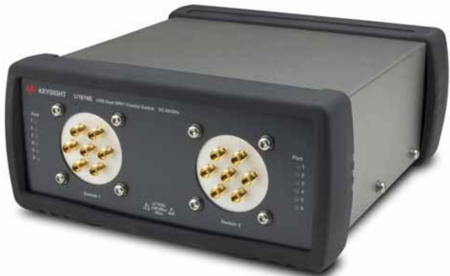
Figure 1-1 U1816x USB-Controlled Switch Matrix
