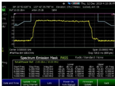
SEM measurement of 5G NR FR1 signal
