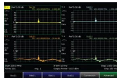
Characterized common and differential mode reflections with mixed-mode S-parameter measurements
