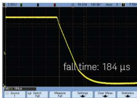
Figure 5. Interrupt pulse fall time measurement of < 200 \mu s
