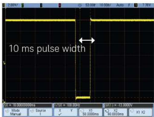
Figure 4. Voltage interrupt pulse generated by N7951A
