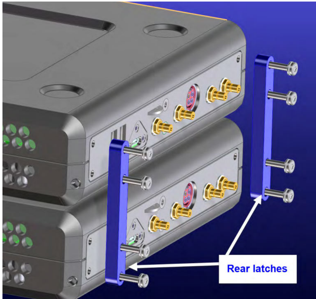
Figure 1-7 Assemble rear latches and screws (0515-0664 screws (x8) and P9375-20018 rear latches (x2)
