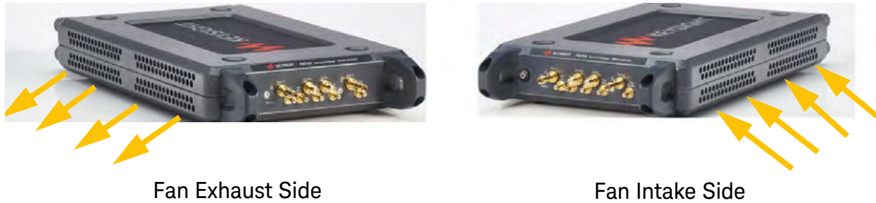
Figure 1-2 P937xA chassis air flow
