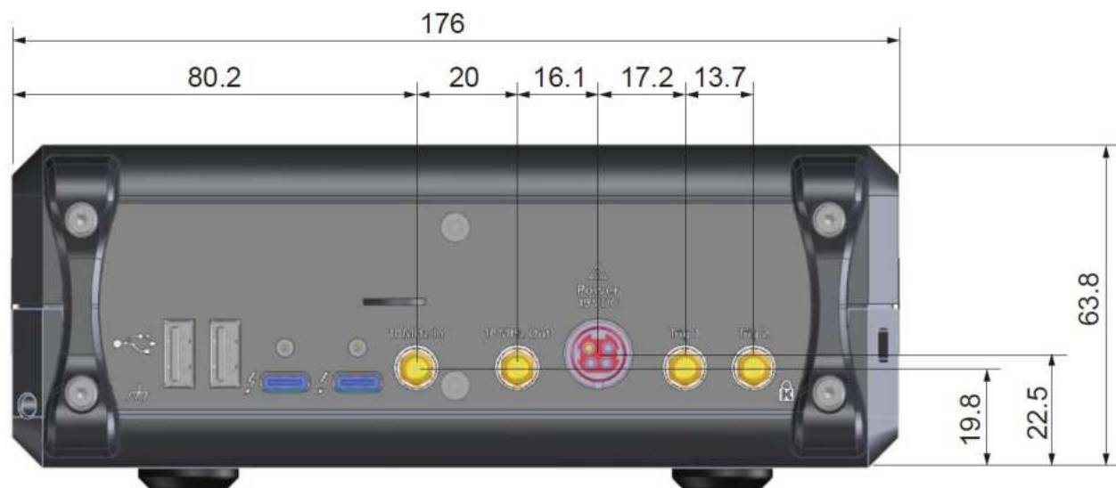
Dimensions (rear view, P5020B/21B/22B/23B/24B/25B/26B/27B/28B with option 400 or 402, or P5020B/21B/22B/23B/24B with option 600, in millimeters)
