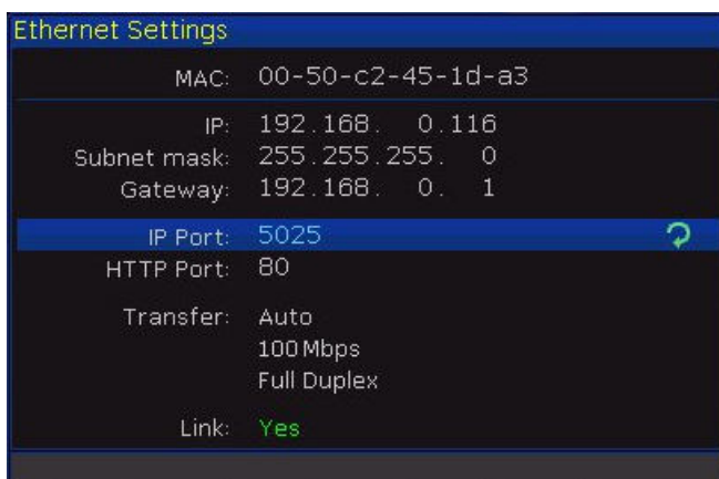
Fig. 3.1: Ethernet settings HMO3000 series
