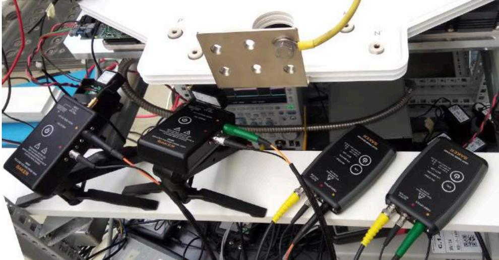
Two ISOVP probes with x10 attenuators measuring IGBT gate voltages in a medium voltage multilevel inverter. Note the use of tripods in the probe heads (client provided image)
