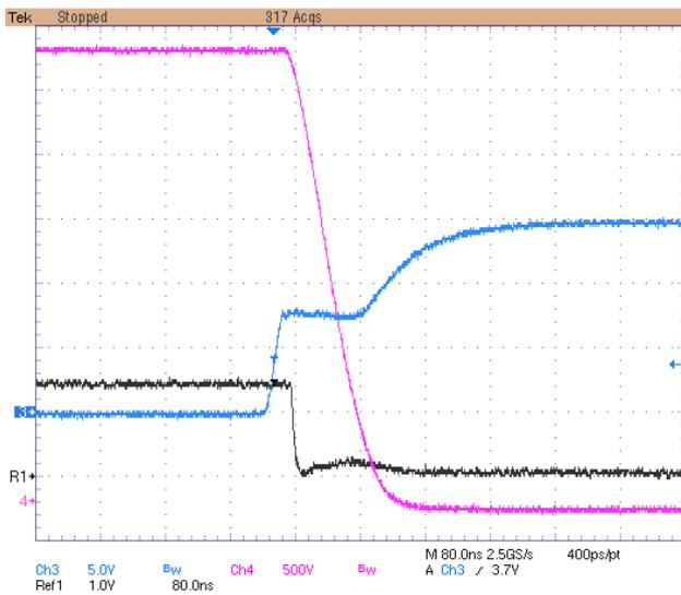
Falling edge detail of Mosfet drain. CH3: Mosfet Vgs.
