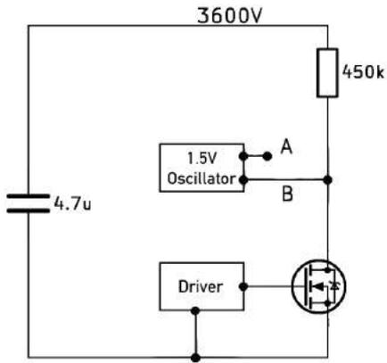
Test circuit for generating fast varying medium voltage common modes. Measuring a 1.5Vpp signal riding in a 3.6kV voltage presents a challenge for any researcher. Oscillator and driver are not in sync.
