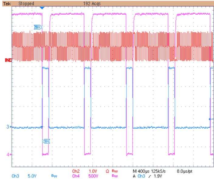
Test circuit measures. CH2: 1.5V oscillator output (A-B) measured with ISOVP probe. CH3: Mosfet Vgs. CH4: Mosfet Vds
