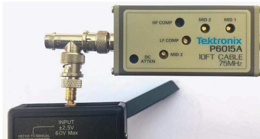
Connection of a 1000x probe through a BNC T. Other types of probes can be connected in the same way. The additional BNC port can be used to add extra compensation capacitance in case the probe needs it.
