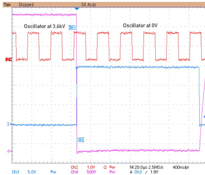
Detailed view of switching pulse. To the left of the CH4 falling edge, the oscillator (CH2) is floating at 3.6kV and at nearly 0 to its right. Such a low voltage measurement is nearly impossible to make with a differential probe given the high common mode of the signal, noise
