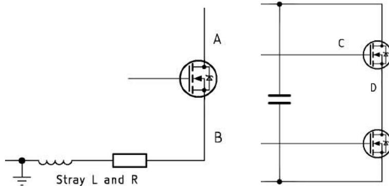
A to B measurement will be greatly affected by high currents and pulsed voltages by stray L and R if taken as a ground referenced measurement. High side gate voltage C to D measurement is typical in power electronics and will need a properly rated probe not only for that particular common mode voltage but also for the switching speeds created by the low side MOSFET.
