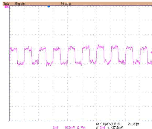
10kHz 10mVpp signal fed into ISOVP probe with oscilloscope into Hi-Res mode
