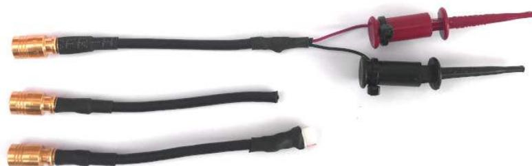
Top and middle: SMB cable with mini-grabbers and unterminated SMD cable (included with the ISOVP probe). Bottom: customer adaptation of an SMB to 2,54mm straight pin cable
